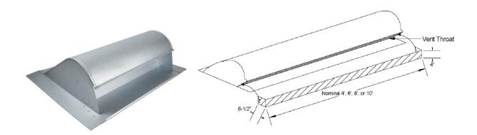
TAMCO Round Top Off-Ridge Vent with Baffle for Tile Minimum 26 ga. ASTM A792 AZ50 (non-HVHZ only) or ASTM A653 G90 galvanized steel off-ridge static roof ventilator with intake baffle for use with low-profile tile roof systems. Vent dimensions are 24" wide x 4-1/4" high and is available in nominal lengths of 4-ft, 6-ft, 8-ft and 10-ft. Material shall conform with FBC Section 1507.4.3 (non-HVHZ) and 1517.6 (HVHZ).
